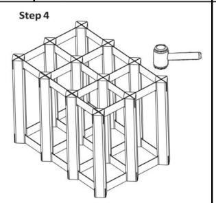
Insert the second section of the metal frame into the first and using a rubber mallet complete the installation into the wood pieces.
