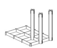
Line up and insert the wood rack pieces into the metal frame. Use a rubber mallet to install into the metal cross frame. Repeat until all wood rack pieces are installed.
