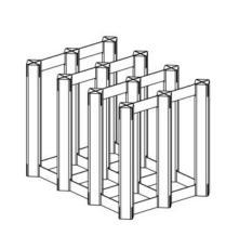
Very important! Insert one section of the metal frame only half way down into the wood pieces.
